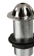
DC Pipe Interrupter For use with urinals and direct flush urinal sensors (to prevent category 5 bacteria contaminating the mains water supply) 15mm inlet, 22mm outlet WRAS approved 46.DCI £85
