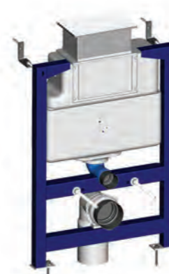
Ancortite 2 in 1 Wall Hung Frame ■ Including pneumatic cistern ■ For use with FP1 and FP2 Flush Plate ■ Adjustment 820 – 1020mm ■ For under window and standard height options ■ Including polystyrene jacket ■ Left or Right turn pan connection option 134.DWC £299
